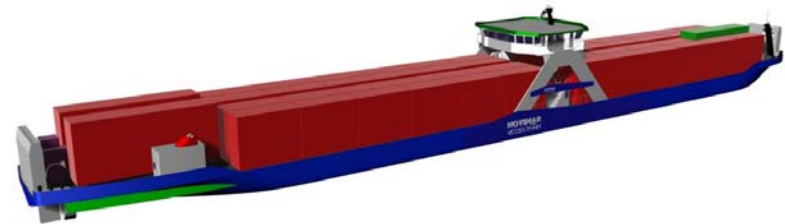
NOVIMAR Class Va, Shallow draft double access Container ro-ro vessel
