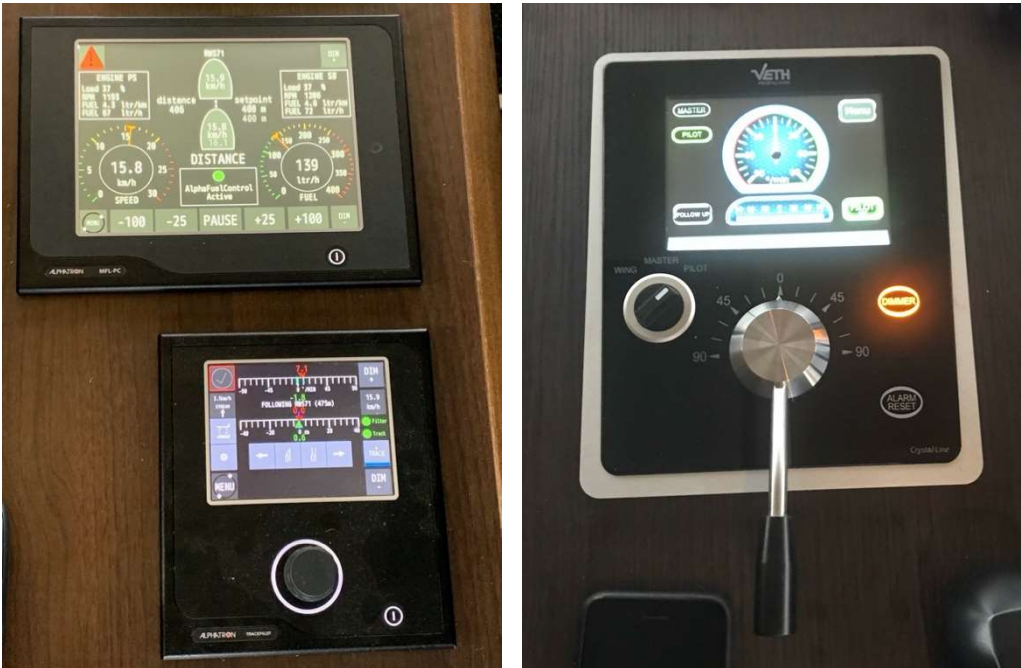
Figure 4: AlphaFuelControl, argoTrackPilot VT and Veth autopilot on the follower vessel
