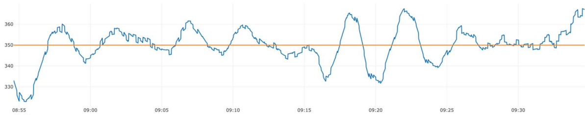
Figure 29: 1 st Run: Longitudinal distance in meters (blue) during experiment with lateral offsets, longitudinal distance setpoint 350m (orange)
