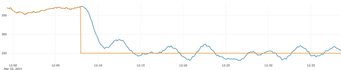
Figure 37: 2 nd Run: Longitudinal distance (blue) and distance setpoint (orange) in meters during experiments with lateral offset. Distance control was activated at 12:07 GMT
