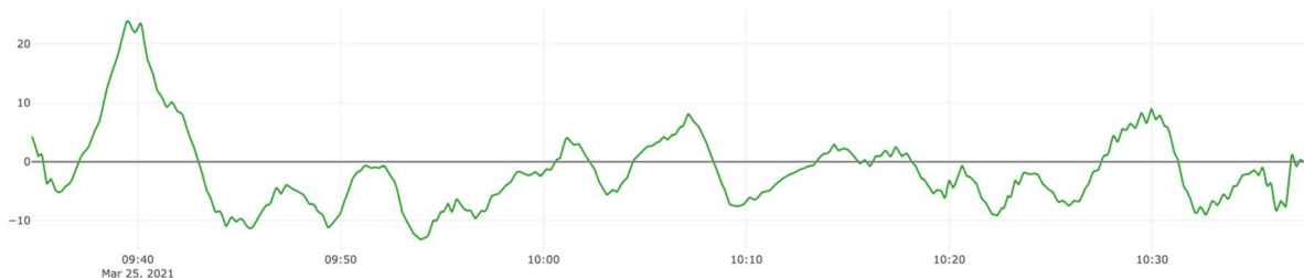
Figure 31: 1 st Run, Distance to track in meters (green) during “assisted guidance”
